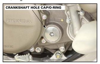
4. Turn the crankshaft clockwise to align the punch mark on the primary drive gear with the "△" mark on the right crankcase cover.
